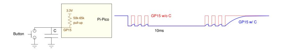
Adding a capacitor filters is one way to remove bouncing
