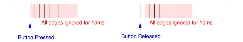
Software Debouncing: All edges are ignored for 10ms once a falling edge is detected
