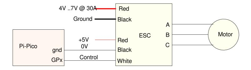
Connections from a Pi-Pico to a BLDC motor.
