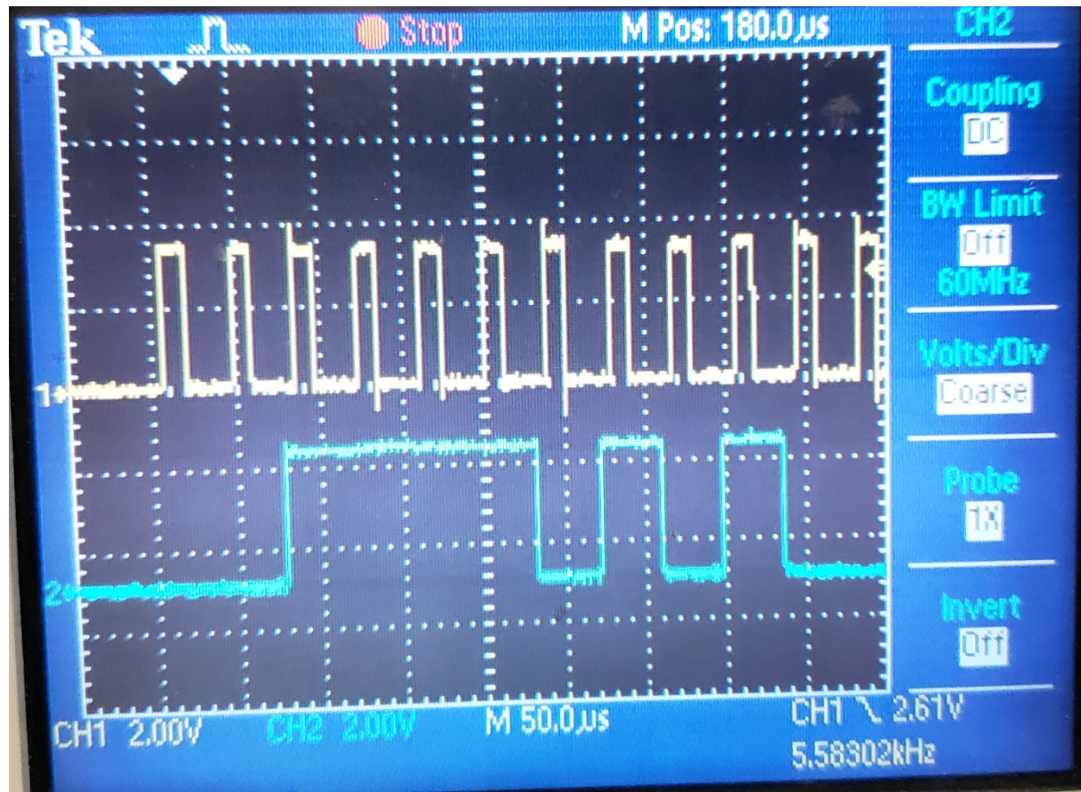
CLK (yellow) and DATA (blue) lines going to the MCP4921 D/A chip
