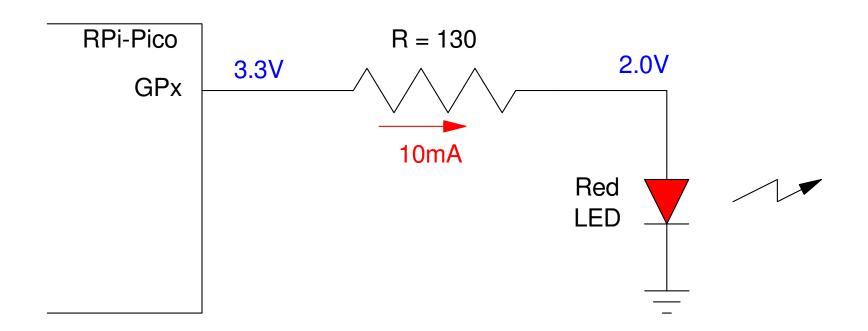
If driving a load that needs less than 3.3V and less than 12mA, you can connect it directly to the RPi-Pico with just a resistor (to limit the current)
