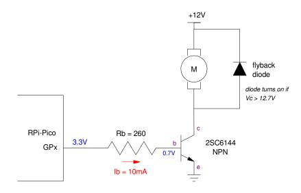
To bleed off the stored energy, the inductor will raise its voltage until it finds a path to ground. With the flyback diode, this voltage is limited to 12.7V
