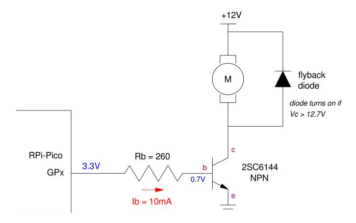
If you are turning on and off an inductive load (DC motor, solenoid), add a flyback diode to limit the voltage at Vc
