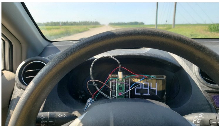
GPS Speedometer: A vehicle's speed is displayed using a GPS module
