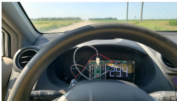
Displaying a car's speed using a GPS sensor
