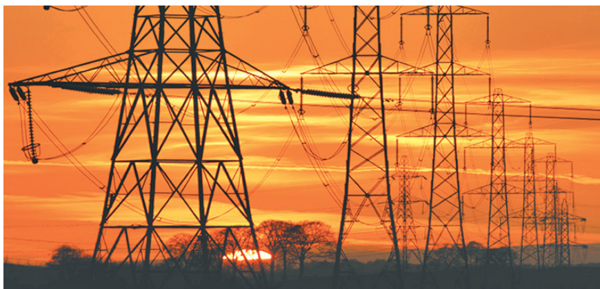
The shape of a hanging chain (or wire or transmission line) is a hyperbolic cosine function
