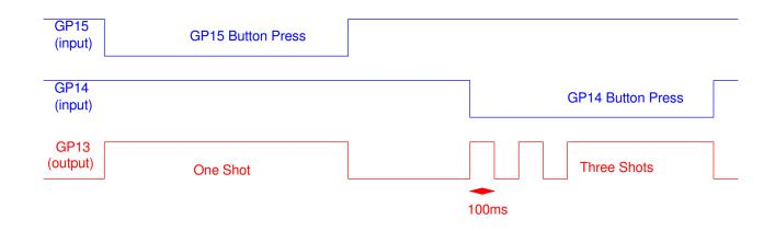
Code: (start with GP14 and 15 are inputs with a pull-down resistor, GP13 is output)
