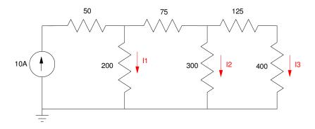
3) Use Thonny as a calculator to determine the voltages {V1, V2, V3}
