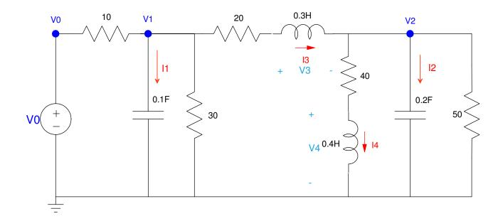
$$I_{1} = 0.1 sV_{1} = \left(\frac{V_{0} - V_{1}}{10}\right) - \left(\frac{V_{1}}{30}\right) - I_{3}$$
