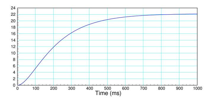
2) Name That System! Give the transfer function for a system with the following step response.
