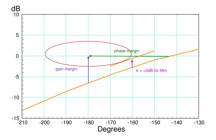
Mm: Pick any point on the m-circle such as  $1 \angle -162^\circ$ . The closed-loop gain is then  $M_m = \left(\frac{G}{1+G}\right) = \left(\frac{1 \angle -162^\circ}{1+1 \angle -162^\circ}\right) = 3.196$
