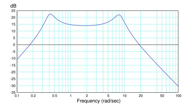
2) Determine the system, G(s), with the following gain vs. frequency
