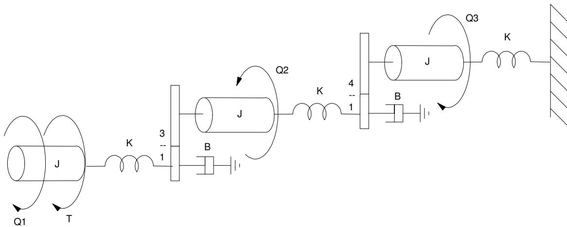
Problem 3:  $J = 2.0 \text{ Kg m} / \text{s}^2$ ,  $B = 0.5 \text{ Ns/m}$ ,  $K = 3 \text{ Nm/rad}$
