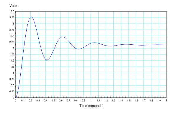
This is a second-order system (oscillations means a complex pole along with its complex conjugate)
