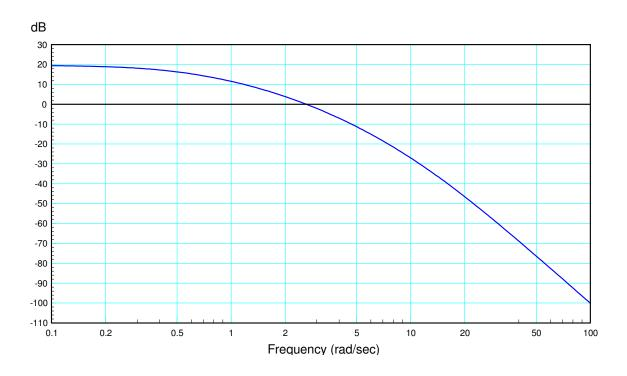
2) Determine the system, G(s), with the following gain vs. frequency
