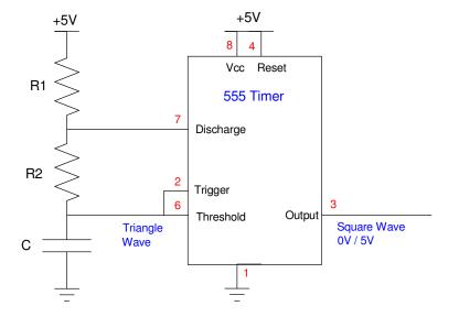
Astable 555 Timer: Problems 5-8 The square wave at the Output has a period of  $T=(R_1+2R_2)\cdot C\cdot \ln(2)$  seconds
