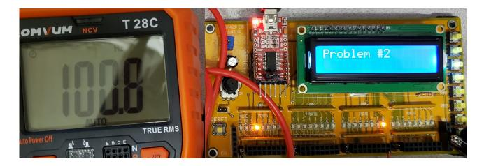
3) Use an INTO interrupt and TimerO to measure the frequency of this square wave (take 1)
