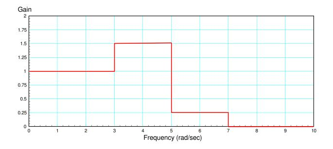
7) Design a FIR filter to approximate this impulse reaponse. Include in your design
