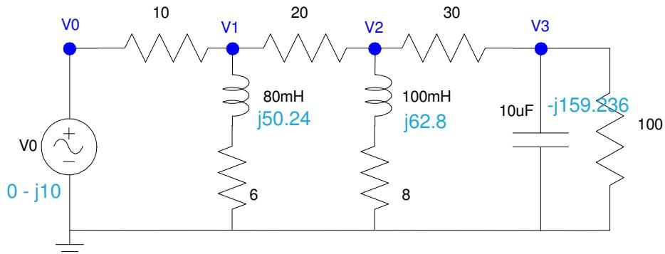
a) Determine the impedances of each element at 628 rad/sec
