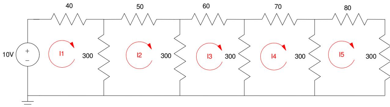
The sum of the volages around any closed loop must be zero
