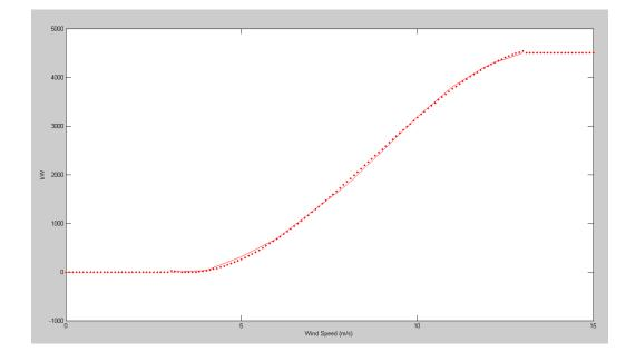
6b) Use this function to compute how much power a Vestas V163-4.5MW wind turbine would produce from the wind data your found in problem 3.
