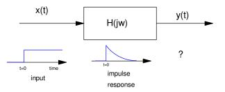
Problem: Find the output of a filter (differential equation) which has an input which is not periodic.
