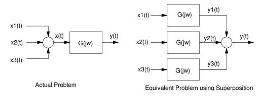
Using Superposition, you can treat a problem with multiple inputs as multiple problems, each with a single input.
