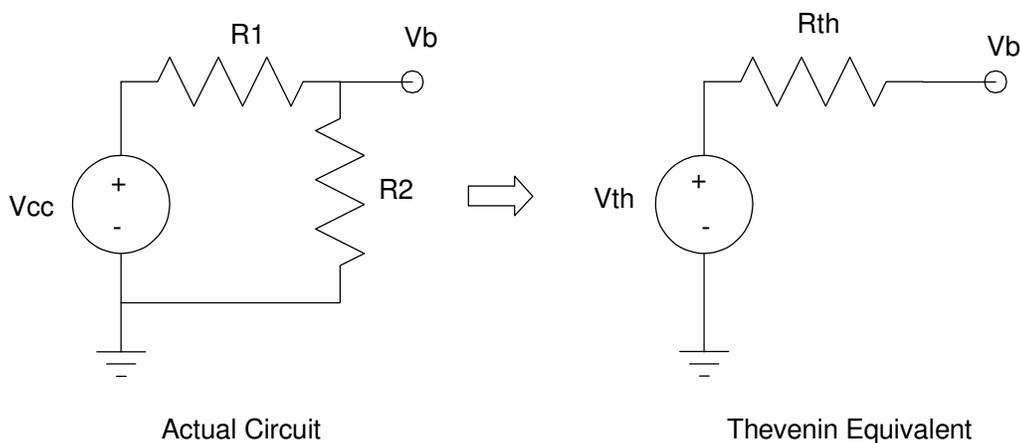
The idea behind Thevenin equivalents is this is a linear circuit: meaning the VI characteristics are a straight line. Any circuit which has the same VI characteristic behaves the same as far as the output is concerned.
