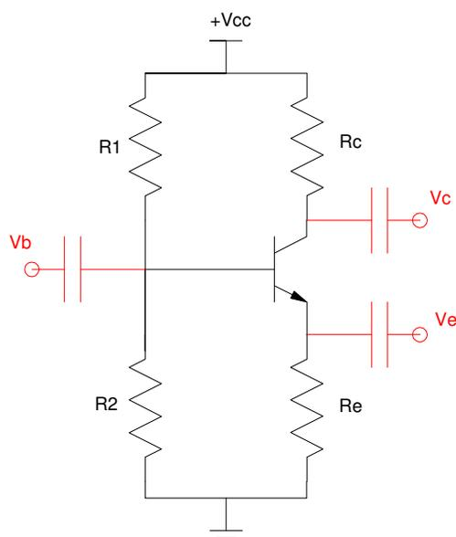
To start, assume  $R_e = 0$ . Taking the Thevenin equivalent of  $R_1$  and  $R_2$ : (One theme in ECE 321 is the use of Thevenin equivalents. You don't have to do this, but if you get use to using Thevenin equivalents, problems in electronics become much simpler.)
