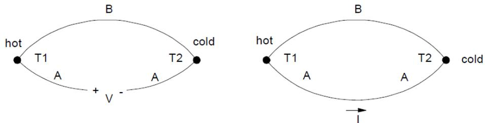
The Seebeck coefficient is a measure of the sensitivity of the thermocouple:
