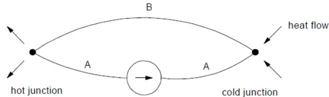
Thomson Effect: If a current is applied to a conductor with a temperature gradient,
