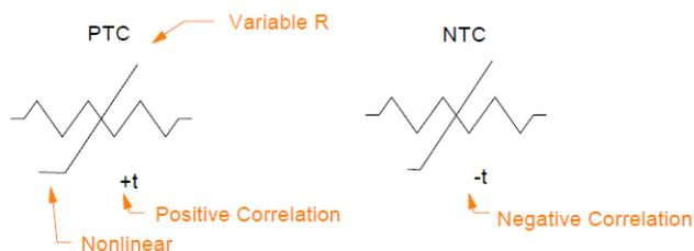
Like the RTD, a thermistor is a resistor designed so that its value changes with temperature. While RTD's are based upon the temperature-dependent relationship of resistance in a metal, thermistors use semiconductors instead.
