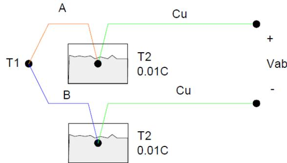
This law allows you to use a third metal in the thermocouple without altering the voltage or current, providing that both junctions are at the same temperature.
