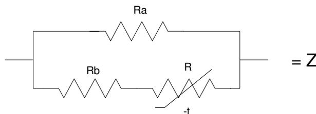
If Ra and Rb are chosen properly, you can sometimes obtain an overall resistance which is linear at two temperatures and the midpoint. For example, if you are using a thermistor with
