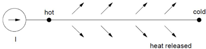
Seebeck Effect: The junction of two dissimilar metals at two temperatures produces a current or voltage proportional to the difference in temperature:
