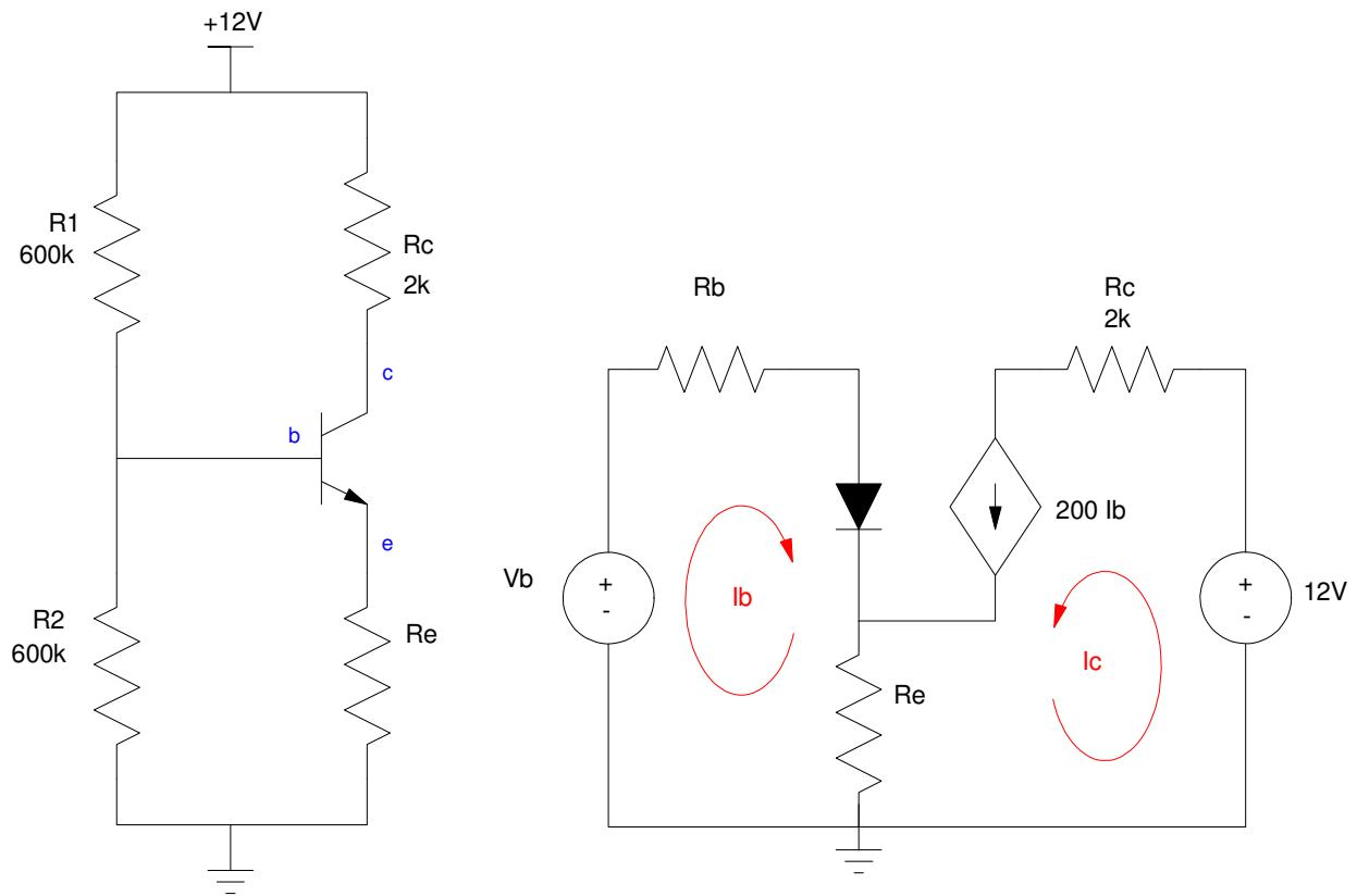
$$V_b = \left( \frac{R_2}{R_1 + R_2} \right) 12V = 6.00V$$
