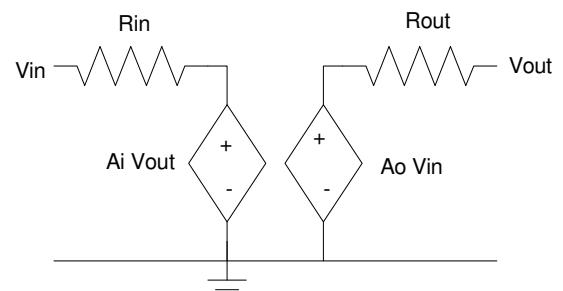
**8. 2-Port model:** Determine the 2-port parameters for a Common-Base amplifier cascaded with a Common Collector amplifier. Assume
