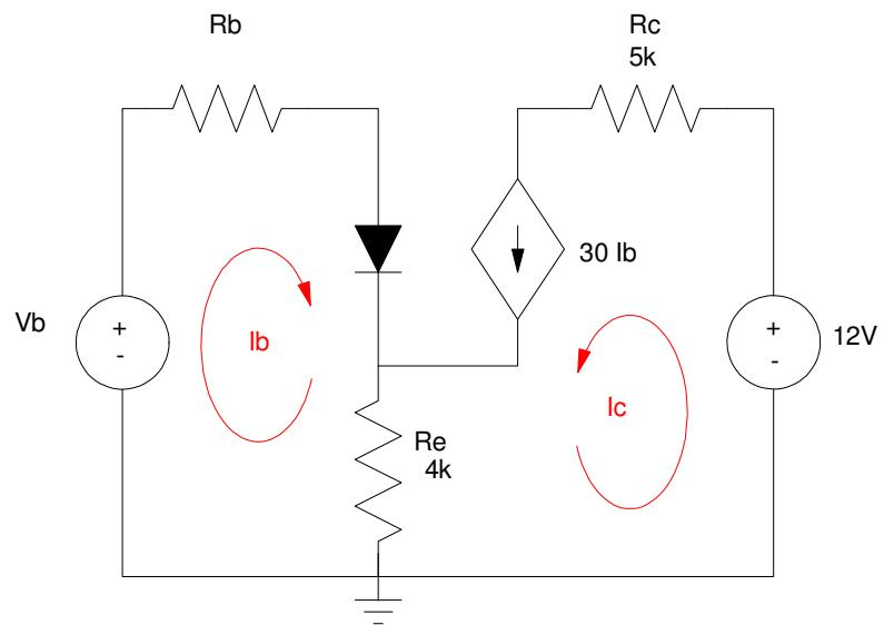
**7. 2-Port model:** Determine the 2-port parameters for the following circuit. Assume
