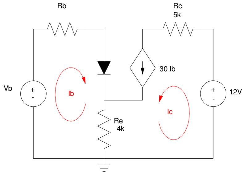
$$R_b = R_1 || R_2 = 1077.9\Omega$$
