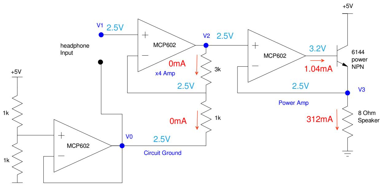
$V_{in} = -0.3V$  relative to circuit ground (2.2V)
