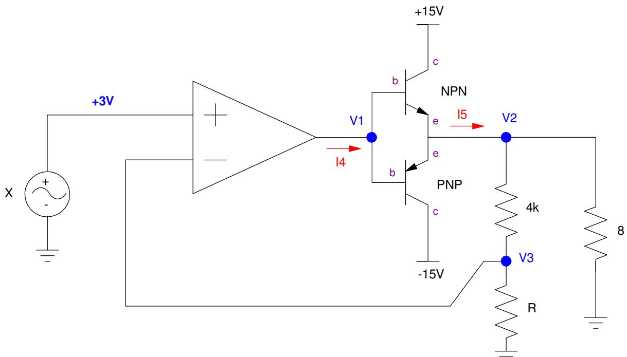
6) Determine the voltages and currents for the following push-pull amplifier. Assume
