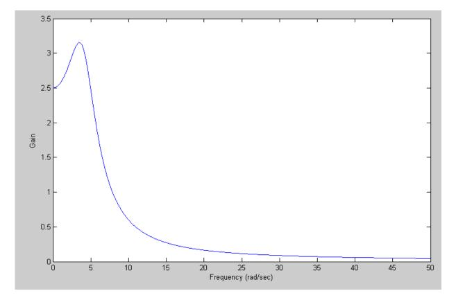
Problem 3-5) Design a filter of the following form so that the gain matches the graph below:
